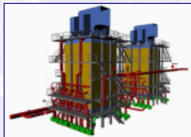
The 3D model in development (PLANT-4D PIPE)
